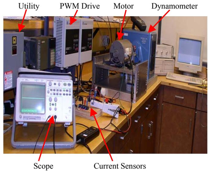
Fig. 4. Laboratory setup of motor-drive system.
