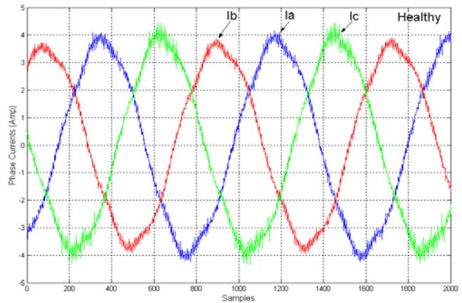
Fig. 5. Stator phase currents under healthy condition.
