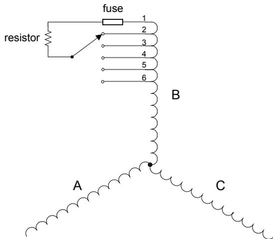
Fig. 2. Schematic diagram of stator windings with taps.
