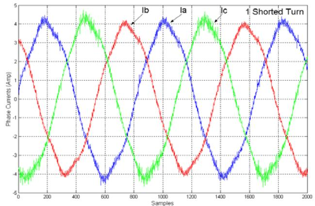
Fig. 6. Stator phase currents under one shorted turn condition.
