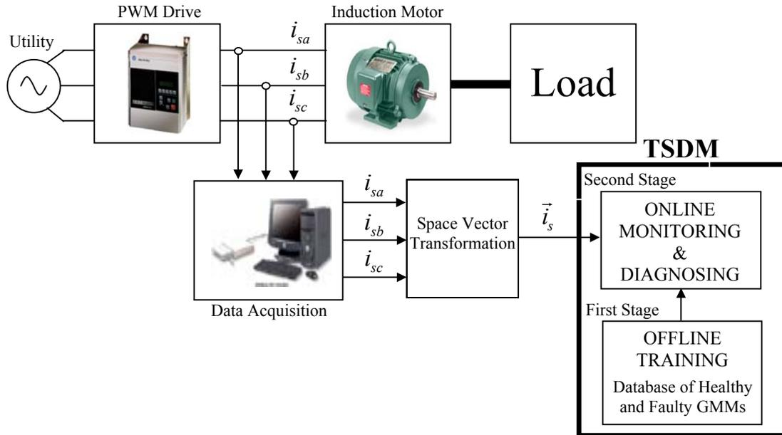
Fig. 1. Block diagram of TSDM diagnostic process.
