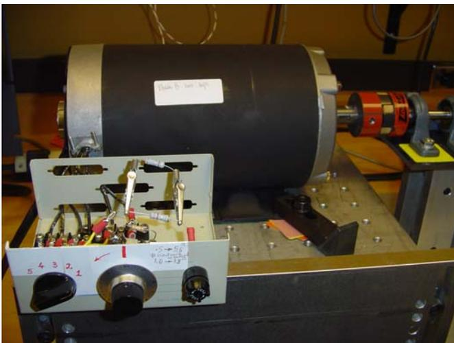
Fig. 3. Actual motor with tapped winding.
